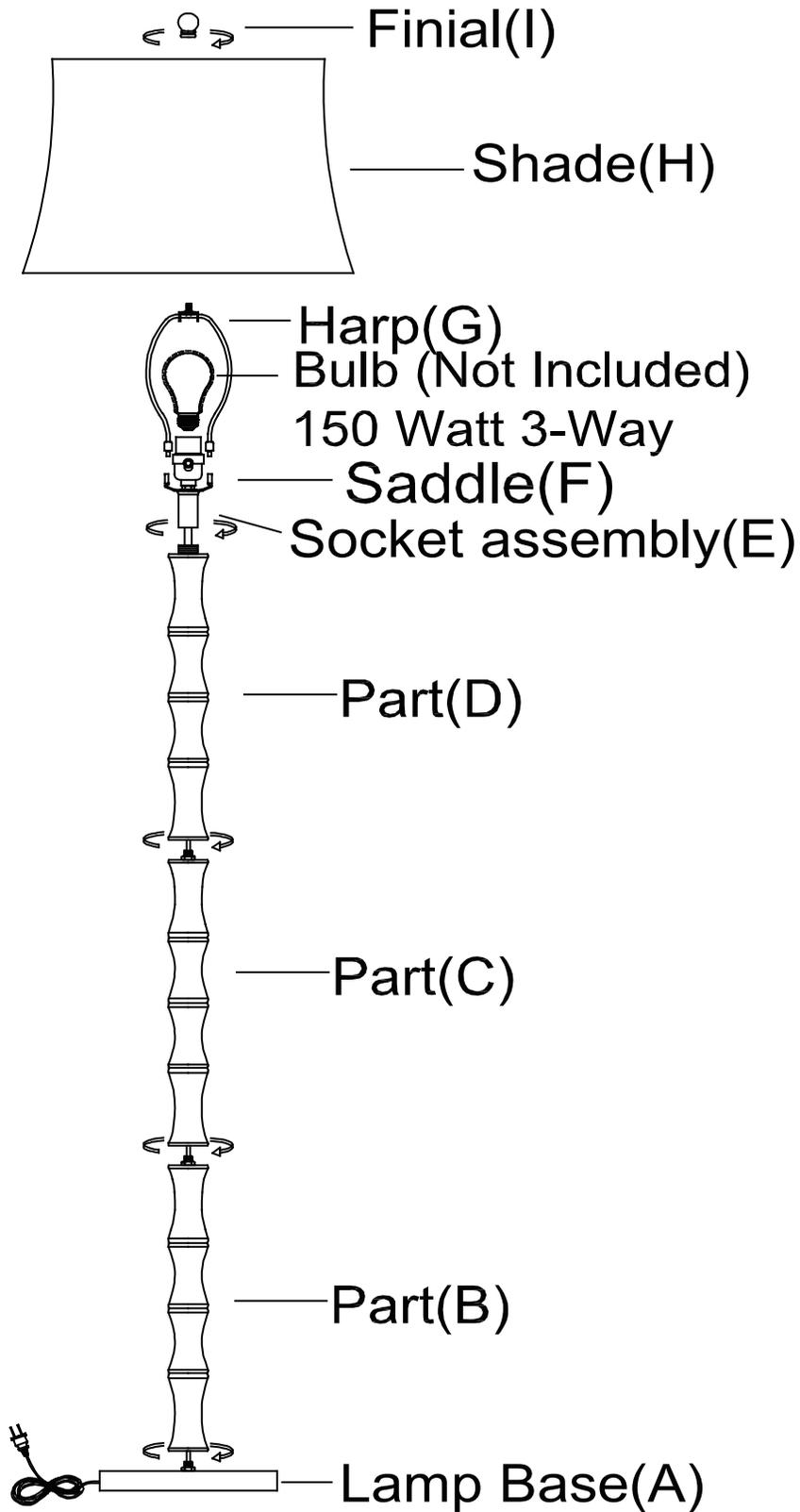
1. Fasten Part (B) onto lamp base (A). Be careful not to twist power cord. Tighten securely.
